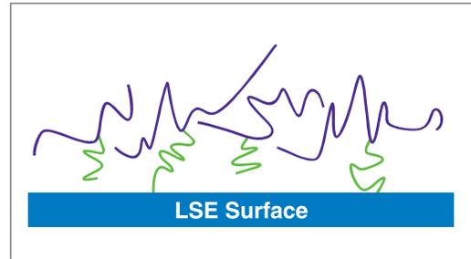
Rubber side chains move down to the surface upon adhesion to a plastic substrate. This starts happening after a few minutes. The adhesion has noticeably increased after 15 minutes and has reached its maximum power within a few hours.
