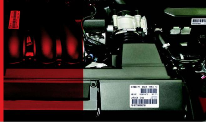
Over the last few decades, there has been an increased use of low surface energy plastics in the automotive, appliance, HVAC, lawn and garden, and industrial segments. Pressure-sensitive label materials with current adhesive technology do not perform adequately with regards to adhesion. They also are difficult to convert and in many cases exhibit adhesive ooze.
