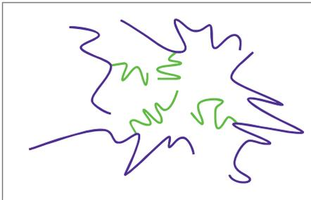
Rubber side chains cluster together inside the adhesive layer and "hide" the rubber properties inside the acrylic backbone. Adhesive appears like an acrylic and is easy to die-cut.
