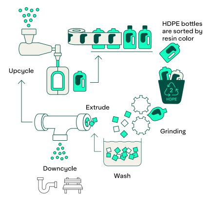
In the second step, HDPE bottles and containers are sorted and washed to help reduce contamination.
