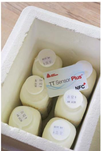
In each shipment a TT Sensor Plus was placed inside of the container and one on the outside in order to monitor the temperature of the product and the outside environment.
