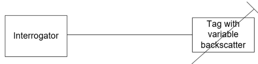
Figure 15b: Conducted test set up for receiver sensitivity with (emulated) tag with variable backscatter
