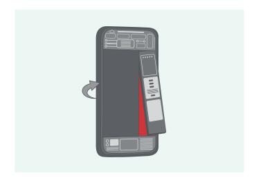
Avery Dennison Performance Tapes has a wide range of high performance pressure-sensitive tapes for mounting and securing components within mobile devices and electronics. Used for battery attachment, Flexible Printed Circuit (FPC) bonding, camera mounting and a range of other components. These tapes offer high adhesion, and help provide stability for delicate components.
