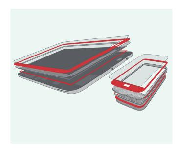
Avery Dennison Performance Tapes offers a range of highly engineered foam tapes designed to meet multiple performance level demands in lens bonding applications. These tapes provide excellent impact, push-out and adhesion performance for mounting display lenses or attaching LCMs (liquid crystal modules) and BLUs (back light units) in smart devices.
