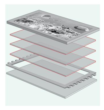
A range of light blocking black PET tapes designed for the bonding and assembly of LCD modules. Bonds well to most LCD components including reflectors, light guide plates, diffusion sheets and brightness enhancement films. These tapes offer multiple performance levels with varying degrees of temperature resistance and light blocking performance (up to 0% light transmission without pin holing per ASTM D1003)
