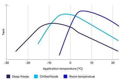
Once in use, our standard adhesives can withstand temperatures from -20 C to + 80 C. Label printers and brand owners can further expand this range by utilizing pressure-sensitive adhesives beyond typical service temperatures, such as:
