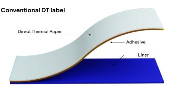
A PS label containing a sandwich structure of liner plus silicone coating with an adhesive layer and facestock
