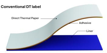
A PS label containing a sandwich structure of liner plus silicone coating with an adhesive layer and facestock
