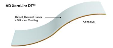
A PS label with a self-wound structure, eliminating the need for a silicone-coated release liner
